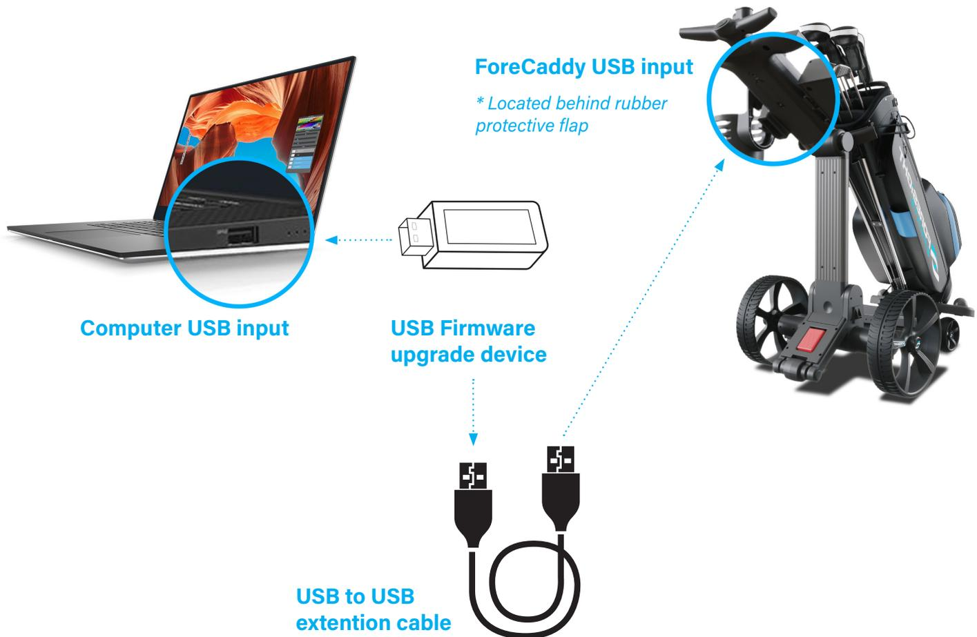
*Note: Firmware upgrade 5.0 requires you to use the USB Firmware upgrade device and connect it to your ForeCaddy via the USB to USB extension cable. Firmware upgrade 5.0 does not require you to upgrade the remote control.*
